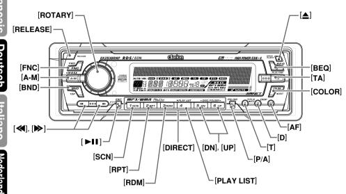
With the SLOPING CONSOLE opened / Ouvrez la CONSOLE RABATTABLE ÖFFNUNG DER SCHRÄGKONSOLE / Apertura della CONSOLE INCLINATA Met het KANTELEND BEDIENINGSPANEEL geopend / Apertura de la CONSOLA INCLINABLE DEN LUTANDE KONSOLEN öppen / Com a CONSOLA INCLINÁVEL aberta
